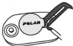
2. Remove the old battery from the battery cover with a suitable sized small rigid stick or bar, such as a toothpick. A non-metal tool is preferable. Be careful not to damage the battery cover.
