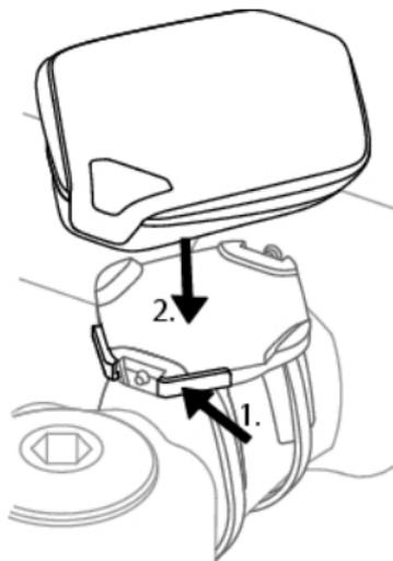
**To detach the cycling computer from the bike mount**, push the button and lift the cycling computer off the bike mount.
