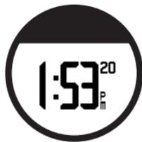
While in power save mode, you can view the time of day, turn on the backlight, and use the ANT+™ computer connection. To exit power save mode, press the **enter** or **quit** button.
