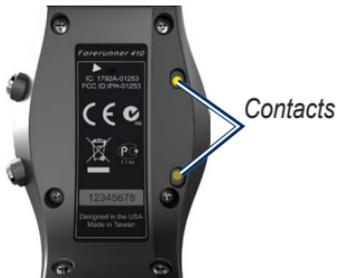
4. Clip the charger securely over the face of the device.
