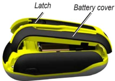
2. Insert the battery. Align the + (positive) and - (negative) markings on the device with the battery.
